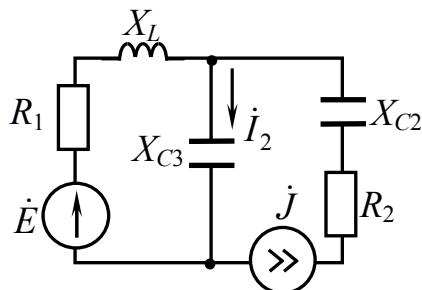
$$\begin{aligned} X_L &= X_{C2} = 10 \text{ Ом} \\ R_1 &= R_2 = 10 \text{ Ом} \\ X_{C3} &= 20 \text{ Ом} \\ \dot{E} &= 10 \text{ В} \\ J &= 2 \text{ А} \end{aligned}$$
